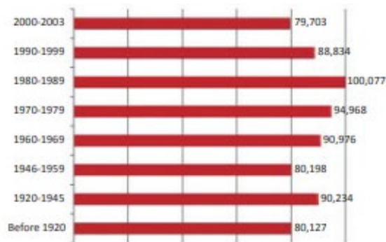
Average Annual Energy Consumption in BTUs (British Thermal Units), commercial buildings. (US Energy Info. Agency, 2003)
